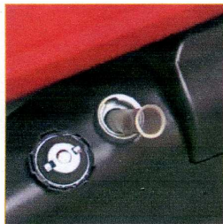
Filtro riempimento serbatoio gasolio Filler filter for fuel tank Cod. 02AC556
